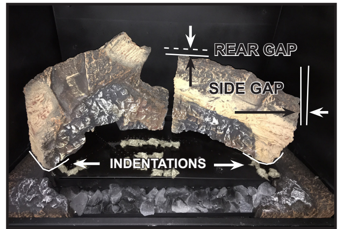
Figure 5. Rear Right Log Installed
