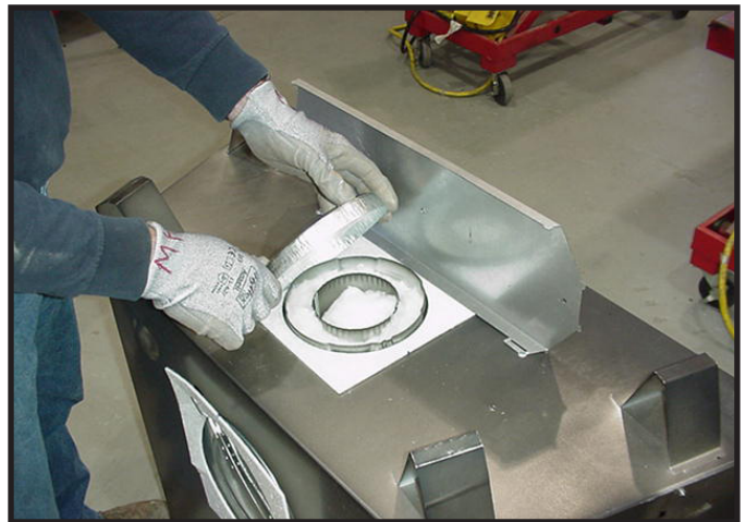
Figure 6.4 Remove the seal cap.
